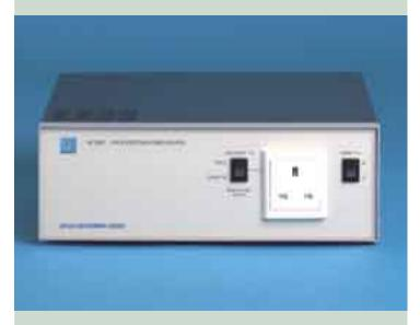
The harmonics standard IEC61000-3-2 specifies that to measure the harmonic performance of a product, a pure, harmonic free supply should be used. Generally, the public mains supply will not meet the requirements of this standard. The AC1000 uses innovative techniques to correct the incoming mains supply and provide a mains source that complies with the requirements of the standard.
