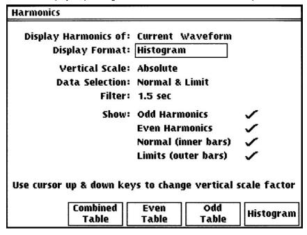
The soft-key functions change as the edit zone is moved through the editable fields of the display using the ▲ ▼ keys; each field is described below. Pressing the VIEW key returns the display to the Harmonics view. The selections made for each of the display formats are stored until the instrument is switched off
