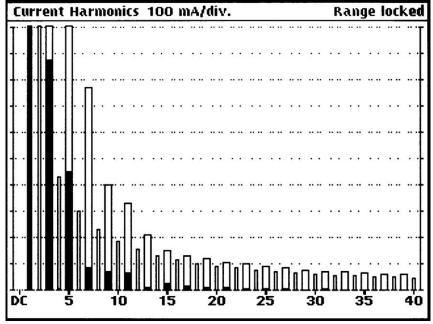
The horizontal scale is marked with the harmonic number. Odd harmonics & limits are shown as wide bars and even harmonics & limits are shown as narrow bars. The fundamental is shown to the left of the second harmonic as a wide bar and the DC component is shown to the left of the fundamental as a narrow bar.
