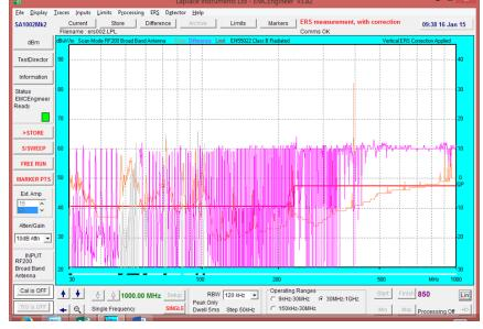
For clarity, the current trace can be switched off to make the difference trace easier to see.
