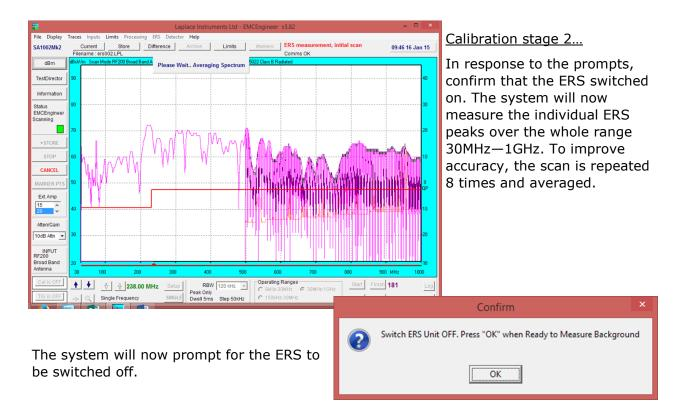
When the ERS is switched off, click OK and the scans will be repeated to check the ambient levels at precisely the same frequencies.
