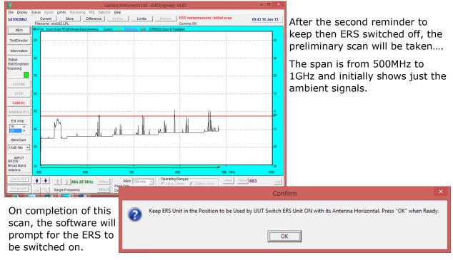
The system will now repeat the scan, displaying the ERS signals. From this scan, the precise frequency of the ERS will be determined. The analyser is now able to precisely measure all the ERS signals from 30MHz upwards.
