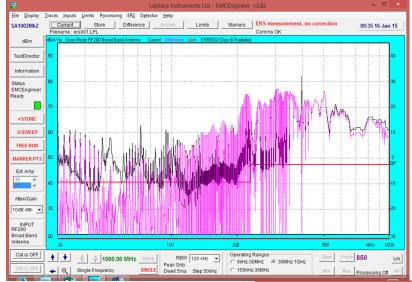
Difference trace switched on. Due to the low levels of ambient, the difference trace closely matches the current trace over most of the spectrum.
