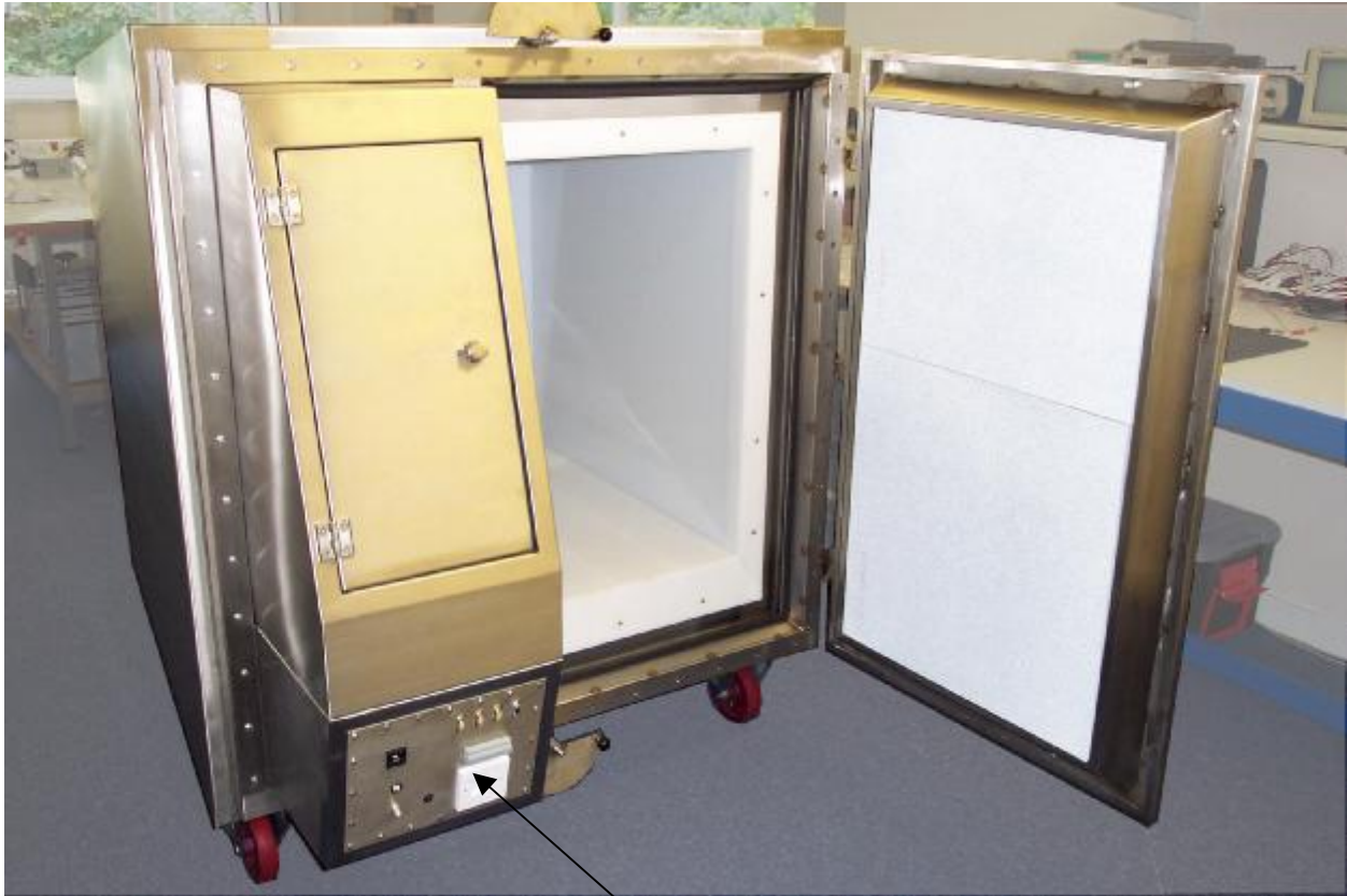
Figure 1 Lower view of rear of cell showing connections to the external world.
