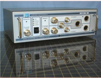
RF Immunity testing above 1GHz normally requires a change of power amplifier. The LETIS system automates this changeover and also provides a connection for a receiver/spectrum analyser so that the system can be switched to emissions measurement mode.
