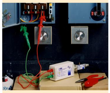
**COMPLIANCE** The PLIP is designed to comply with the CISPR16 requirements for a voltage probe. The design incorporates several features that are in addition to the basic CISPR16 specifications. These offer three major advantages:
