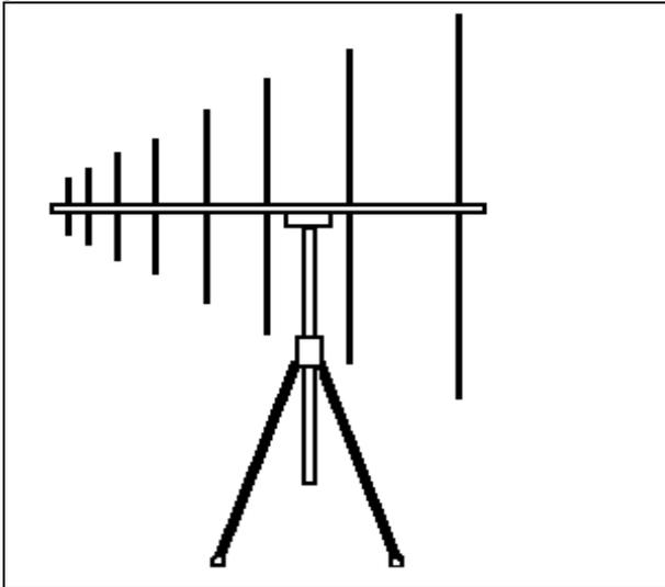
This is supplied as a central vertical support fitted with a leg attachment moulding and three legs.
