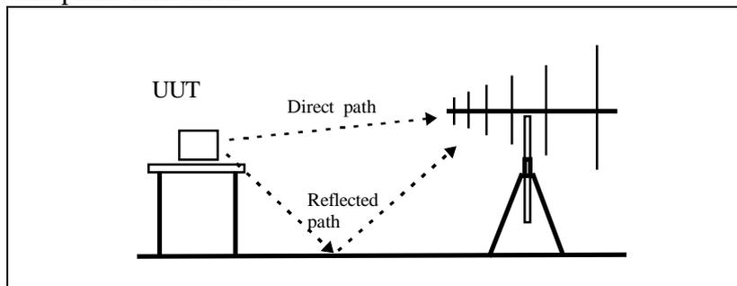
To overcome this effect, the standards call for the antenna to be mounted on a mast so that it can be varied in height over a range of 1 to 4 metres. For each frequency there will be a height at which the two signals are in phase and additive. This is the height at which that frequency is measured.
