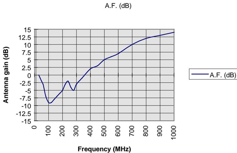
Fig 3(b) RF200 Antenna Factor, Log frequency scaling
