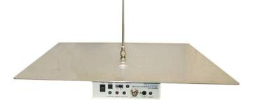
The RF550 Active Monopole antenna is an active, general-purpose, receive-only antenna that covers 9 KHz - 30 MHz frequency range. It is ideal for instantaneous bandwidth scanning (without tuning) of electric fields in its frequency range and can drive any receiver with 50-ohm input impedance. This antenna is an ideal solution to perform FCC, MIL-STD and TEMPEST tests.
