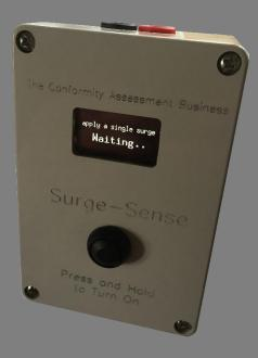
The Surge Sense has been developed with EMC test laboratories in mind to enable a "go / no-go" verification of the surge generator output prior to test. The Surge sense produces an arbitrary pulse length measurement that is dependent upon the surge energy - amplitude and duration, if either of these parameters changes then the pulse length measurement changes. This gives a very quick repeatable check prior to testing and enables simple trend analysis data to be captured.
