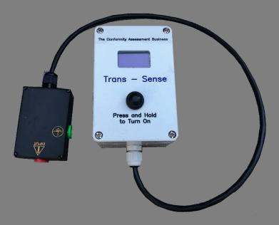
The Trans Sense has been developed with EMC test laboratories in mind to enable a "go / no-go" verification of the transient generator output prior to test. The Trans Sense produces an arbitrary relative amplitude measurement that is dependent upon the applied transient level when measuring 15 / 300 ms bursts. This gives a very quick repeatable check prior to testing and enables simple trend analysis data to be captured.
