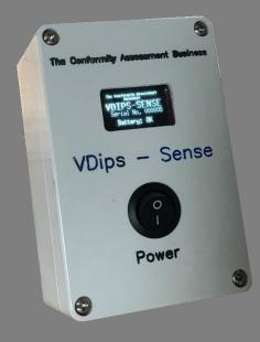
The Vdips Sense has been developed with EMC test laboratories in mind to enable a "go / no-go" verification of the Voltage Dip generator output prior to test. The Vdips Sense measures duration of interruptions on the mains supply from 2 ms up to 20 s. This gives a very quick repeatable check to ensure that the generator is operating as intended prior to commencement of test.
