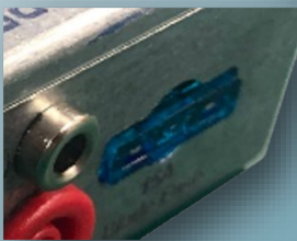
Integrated 15 A automotive blade fuse
